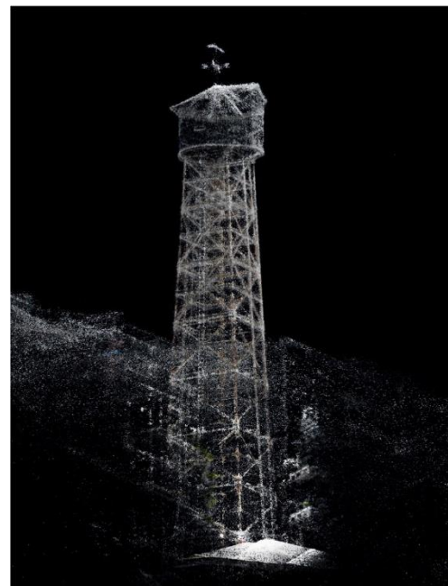
Processed photogrammetry point cloud rendered in RealityCapture (Sam Smith, Woods)
