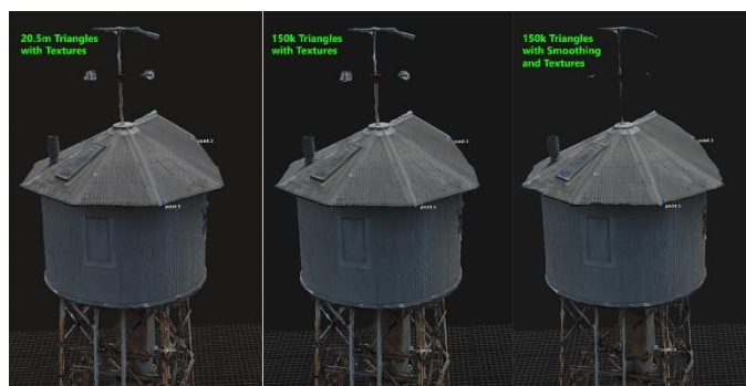
Colonial Ammunition Shot Tower. Comparison of textured mesh model after simplification and texture reprojections. Credit (Sam Smith, Woods)
